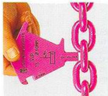
Testing pitch elongation caused by wear of nominal diameter
