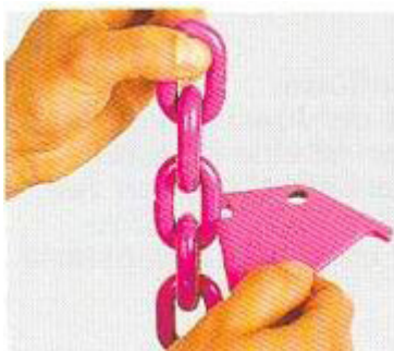
Testing wear of nominal diameter
