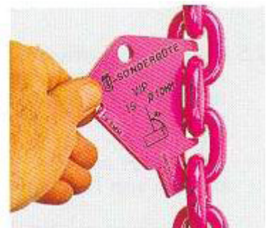
Testing plastic elongation caused by overloading
