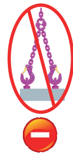
Pic 2: Wrong assembly and usage. Only one load bearing strand is permissible
