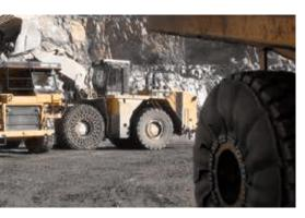
The SIDEFLEX® is a retrofit device for construction and mining equipment, especially for earthmoving machines. The device is mounted to the wheel hub of utility vehicles as dumptrucks or wheel-loaders.
