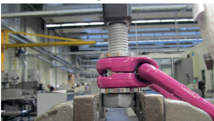
Pic. 8: Dismantling position of the VLBG-PLUS
